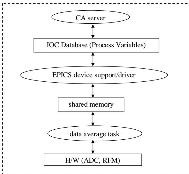
Figure 3: Software structure of the new BPM IOC.
