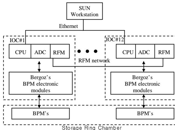
Figure 1: Configuration diagram of the new BPM data acquisition system
