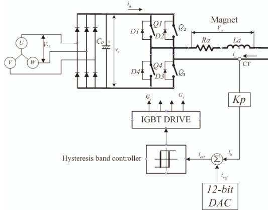
Figure 1: Circuit diagram of the old CMPS.
