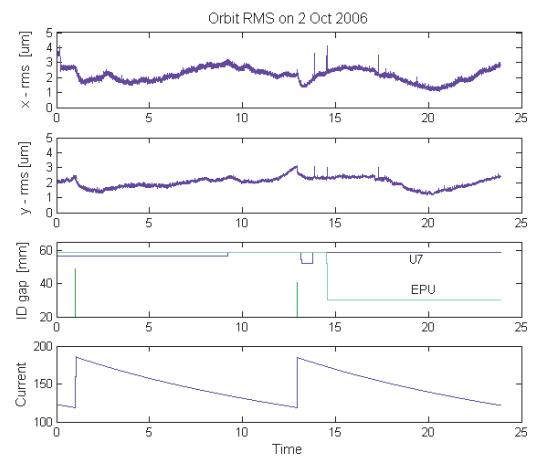
Figure 6: Orbit stability measured for one day.
