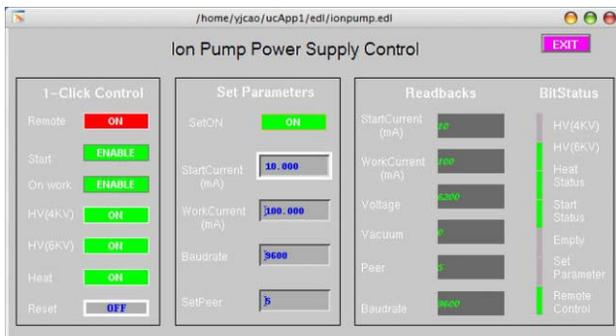
Figure 2: Control panel for JJJ ion pump ps controller.
