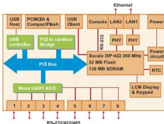
Figure 1: Hardware block diagram of UC7400.
