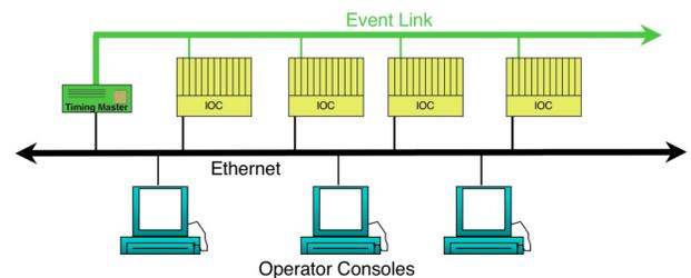
Figure 2: Proposed New System Design With Distributed Timing And Data Acquisition.
