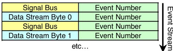
Figure 4: Event Stream Showing Signal Bus and Data Stream Multiplexing.
