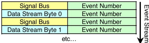
Figure 4: Event Stream Showing Signal Bus and Data Stream Multiplexing.
