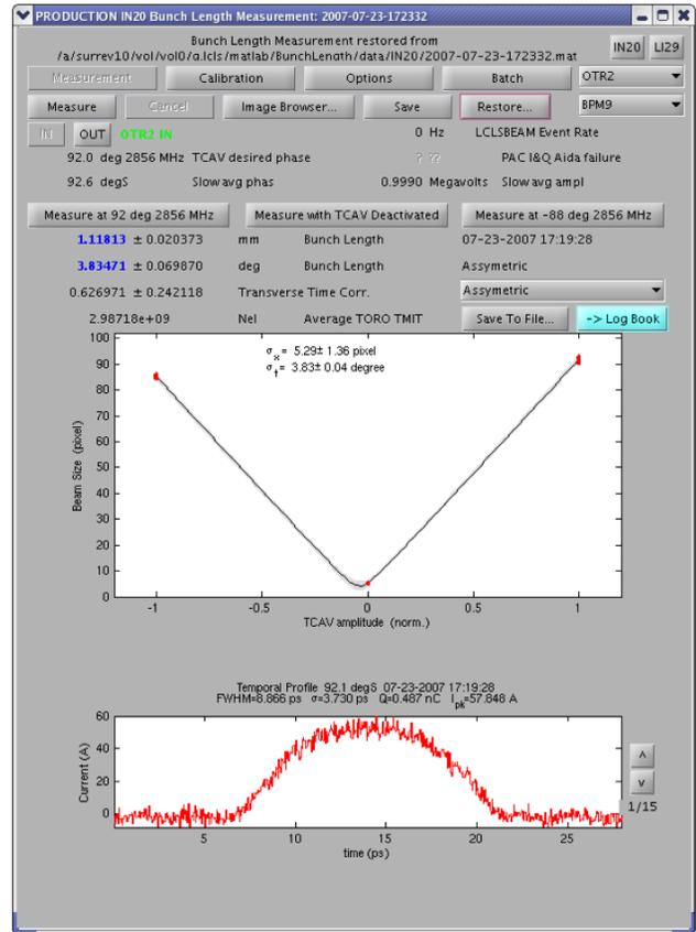
Figure 6: Screenshot of the Bunch Length Measurement application scripted in Matlab, using in Mathwork’s GLIDE tool for constructing graphical user interfaces for Matlab programs.
