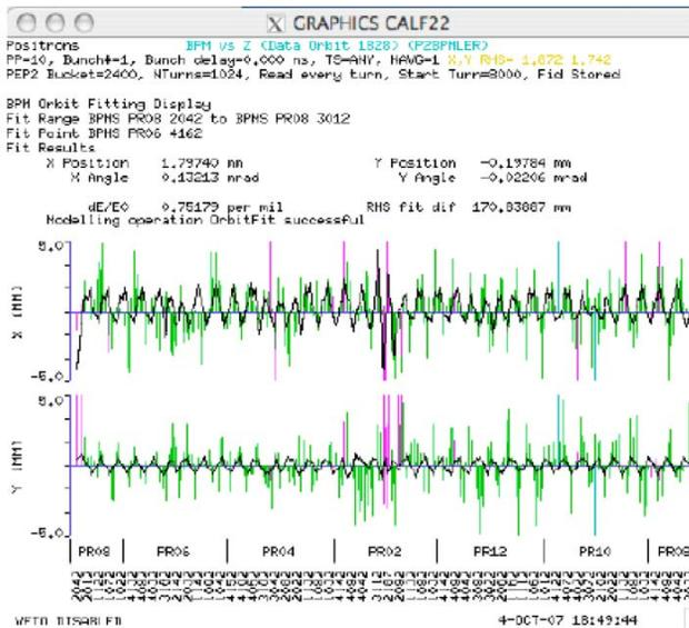
Figure 3: Orbit fitting in the SLAC Control Program. This brings together orbit acquisition, save/restore configurations, and beamline orbit plotting.
