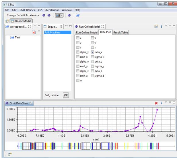
Figure 7: SEAL with the *Online Model* perspective. The perspective contains a workspace navigator displaying the workspace file system (upper left), a beam line sequence selector (upper middle), an online model run control (upper right) and an orbit data plot panel for showing the model run result (bottom).
