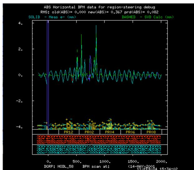
Figure 4: Orbit Correction example from the SLAC B-factory, showing an acquired beam orbit and calculated correction and predicted resulting orbit.
