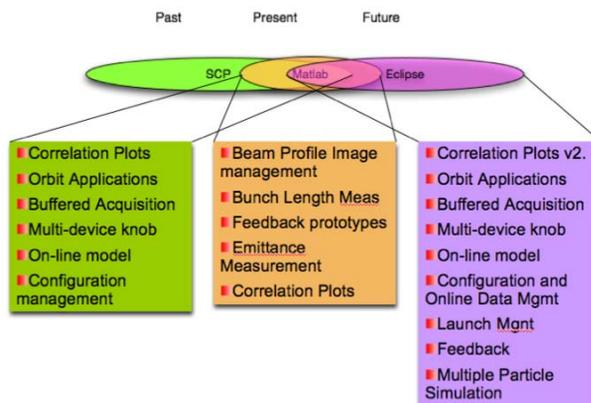
Figure 1: Transitional phase of SLAC online physics software tools. Physics tools are being moved from a legacy Fortran/C VMS system, to Java/Eclipse on Linux; matlab is helping to bridge the gap.
