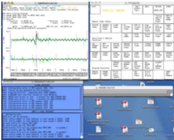
Figure 2: The user interface is composed of 3 main screens: i) a "panel" screen housing all the "buttons" of the Graphical User Interface (there are no pull-down menus, sliders, dials etc), ii) a graphics screen on which all data is presented, mostly in tabular or graphical form, and iii) a continuously updating message window that presents all messages relating to what the individual SCP user is doing in one half, and all global messages of the accelerator in general in the other half.
