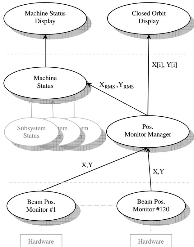
Figure 1: Hierarchical view of the beam position data dispatching.
