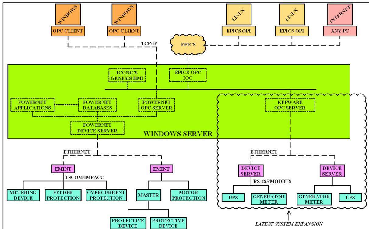
Figure 1: SNS Power Monitoring System Architecture
