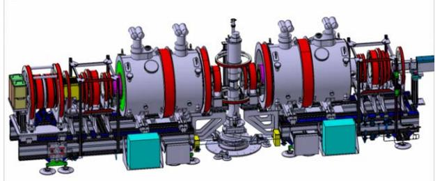
Figure 1: NSE secondary spectrometer; detector is on the left side.
