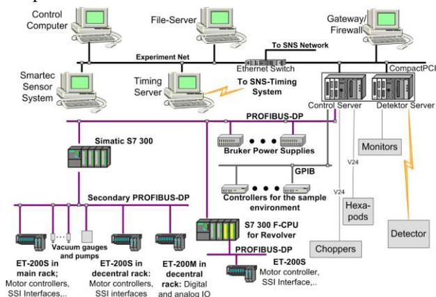
Figure 2: Physical architecture of the NSE control and data acquisition system.
