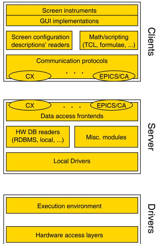
Figure 2: Plugin-based architecture of CX version 4 (shown are pluggable parts).
