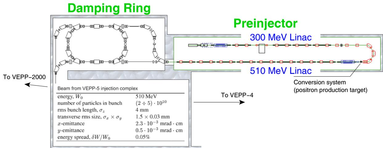
Figure 1: VEPP-5 injection complex layout and parameters.
