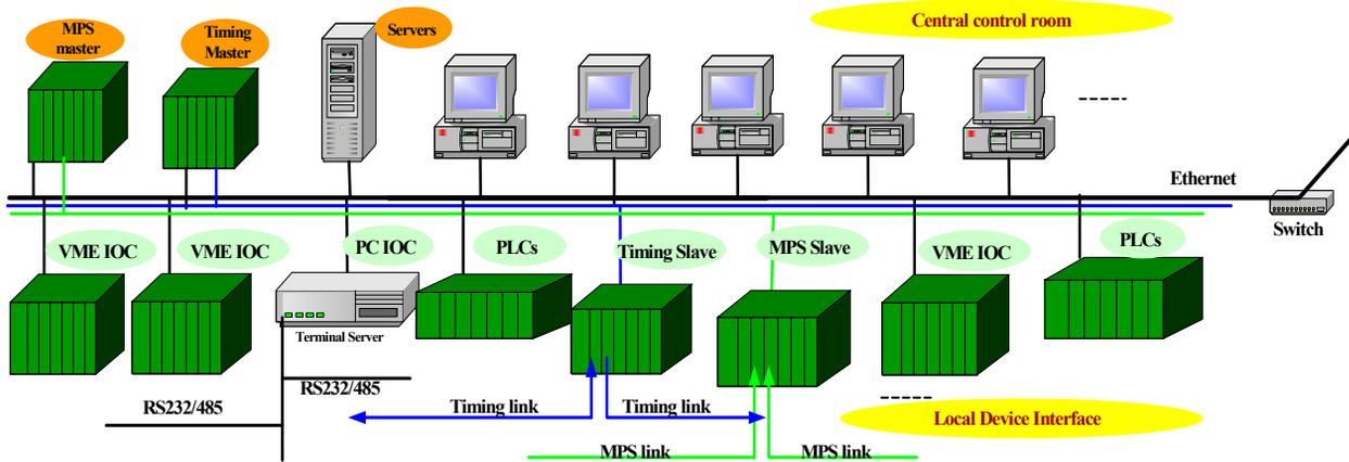
Figure 3: CSNS Controls Architecture
