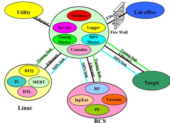
Figure 2: CSNS Controls Scope
