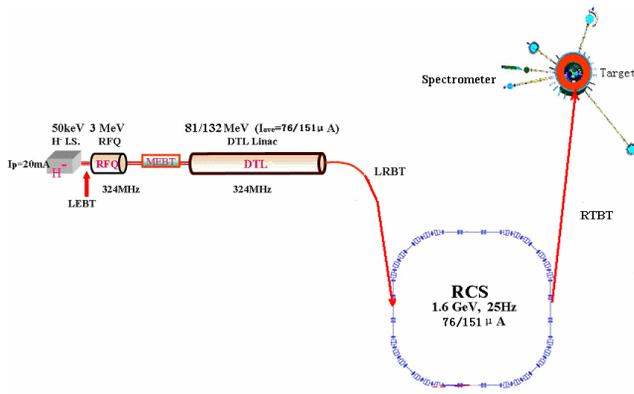
Figure 1: The Schematic Layout of the CSNS Facility
