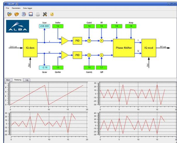
Figure 2: Graphical user interface of the for the low level analogue regulation of the RF. It is written in Python and Qt4.
