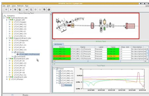
**Figure 5: Graphical interface of the vacuum control of the Linac to booster transfer line.**
