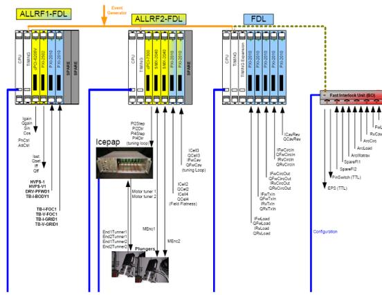
**Figure 3: Block diagram of the control and data acquisition built on top of the low level RF regulation.**
