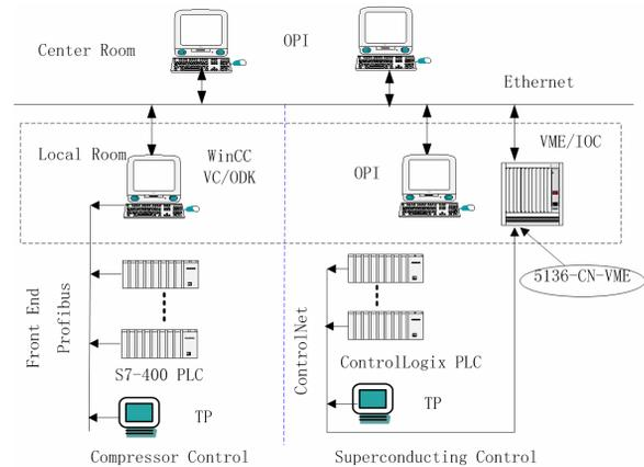
Figure 1: the cryogenic control structure of BEPCII project
