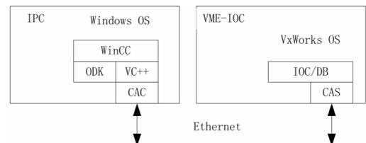
Figure 2: The structure of communication between S7-400 PLC and EPICS IOC
