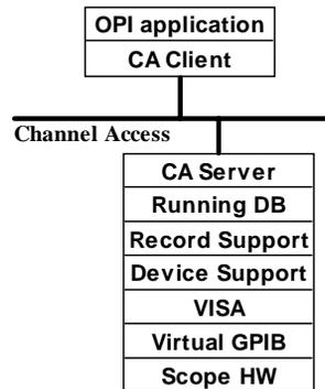
Figure 6: Diagram of Windows scope IOC.
