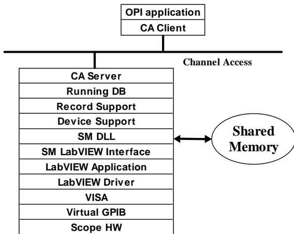
Figure 4: Shared Memory IOCcore interface.
