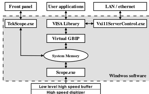
Figure 3: Software diagram of Tektronix scope.
