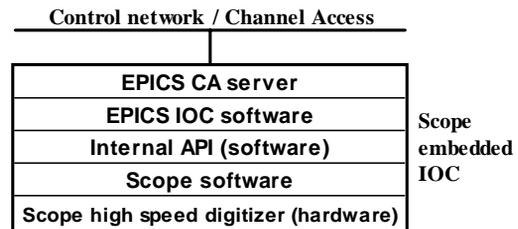
Figure 2: Diagram of embedded scope IOC.
