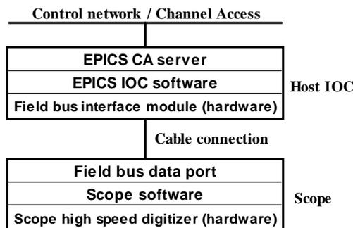
Figure 1: Diagram of a field bus based EPICS scope.
