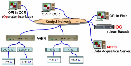
Figure 3: Configuration of Monitor Control using WER.
