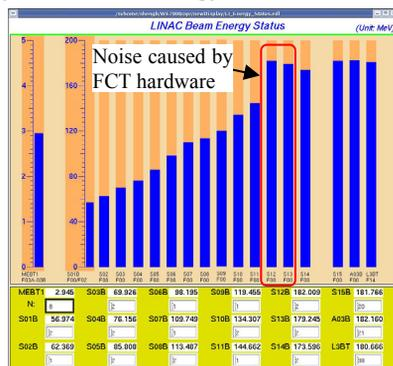
Figure 7: Real-Time Beam Energy Calculated inside IOC.
