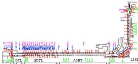
Figure 1: Monitor Device Layout in J-PARC LINAC.
