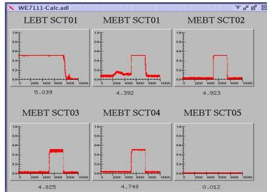
Figure 5: Beam Current Waveform Monitor from SCT.
