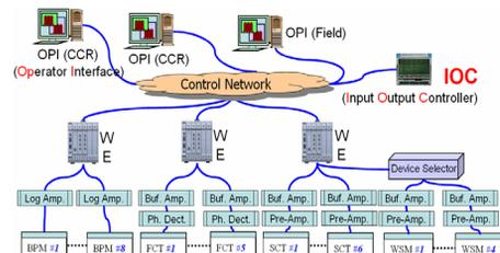
Figure 2: Monitor Control for WE7000 in MEBT1.
