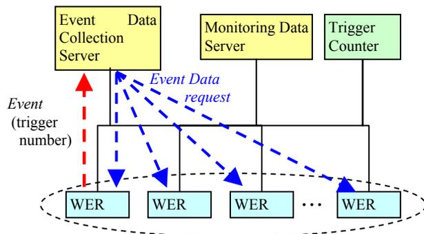
Fig.4 Configuration of WER Acquisition
