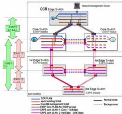
Fig.3 Protocol Configuration for Redundancy of network
