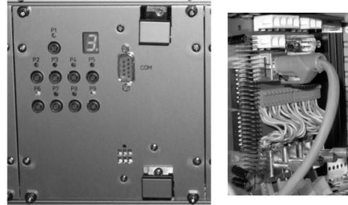
Figure 1: Device Control Unit (front view and rear view with RTB and network cable)
