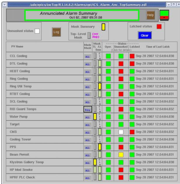
Figure 4: The Annunciated Alarm Summary and the soft IOC that provides its data and functionality is built automatically using the Soft Alarm scripts.
