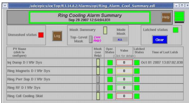
Figure 5: Another automatically created screen, the Ring Cooling Alarm Screen, shows individual alarm status bits.
