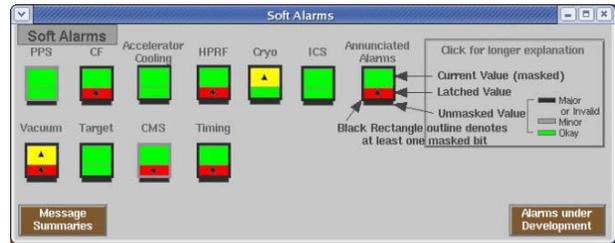
Figure 1: The Top Alarm Summary displays the status of all the alarms in the system. Since EPICS process variables provide the status, the information can be used in any EPICS client application.
