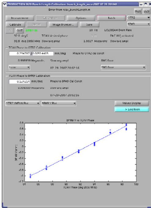
Figure 3: TCAV phase to BPMS y-position calibration
