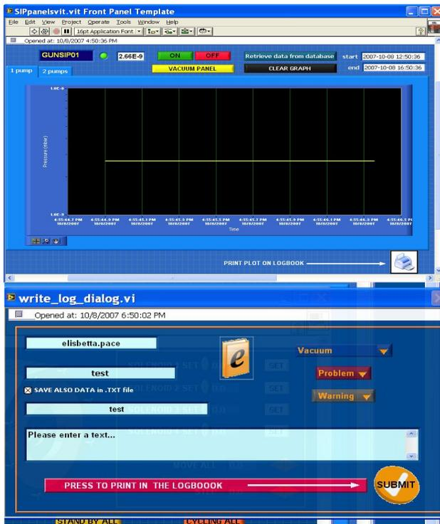
Figure 6: LabVIEW control panel for creating an entry in SPARCbook.
