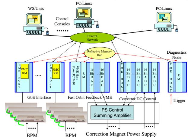
Figure 3: Infrastructure of the new fast orbit feedback system.
