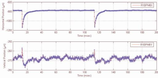
Figure 4: Perturbed beam position due to field leakage of the injection septum.
