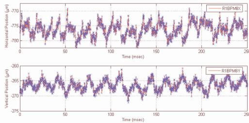
Figure 5: Strong line frequency components appear at the measured beam position.
