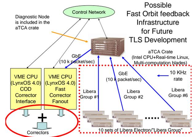
Figure 7: Architecture of the proposed orbit feedback system for further upgrade for TLS.
