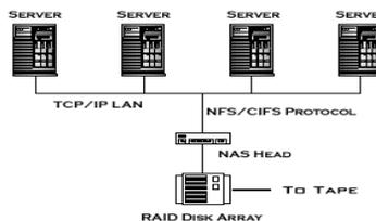
Figure 2: Diagram of typical NAS System.
