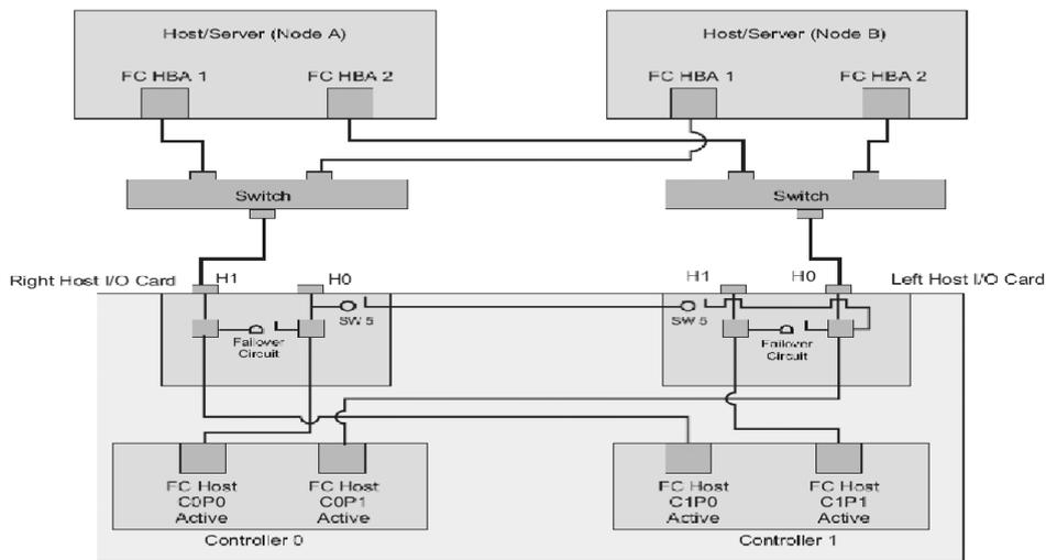
Figure 4: Diagram showing system with redundant paths.
