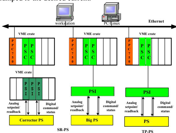
Figure 1: BEPCII PS control system architecture.
