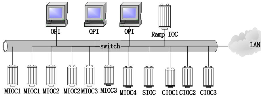
Figure 3: PS IOC Distribution in the network.
