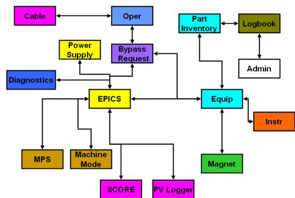
Figure 1. Layout of CSNS database model.
