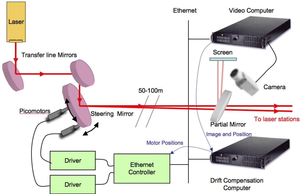
Figure 1. Diagram of the Drift Compensation System.
