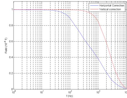
Figure 3: Attenuation of the magnetic field.
