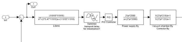
Figure 4: Simulink model of the FOFB.
