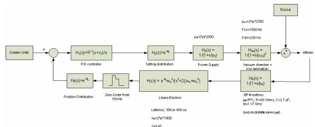
Figure 1: Model of the FOFB correction loop.
