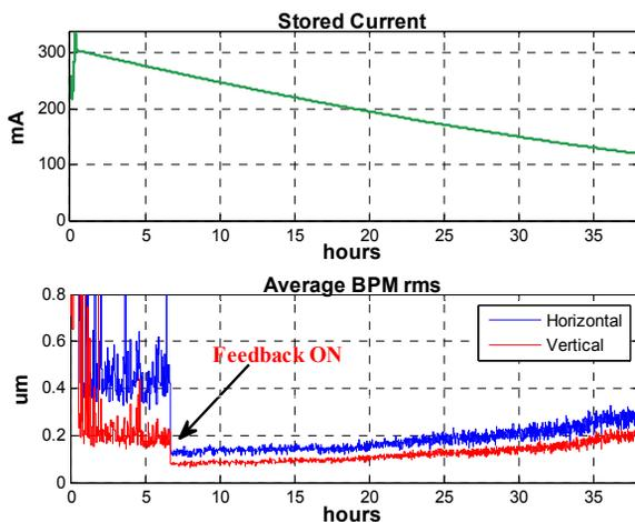
Figure 3: Average beam position *rms* using 10 Hz data of all the BPMs. The feedback is switched on at 270 mA.
