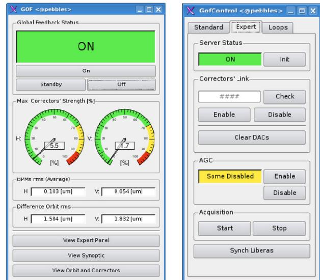
Figure 2: Operator (left) and expert (right) control panels of the fast global orbit feedback.
