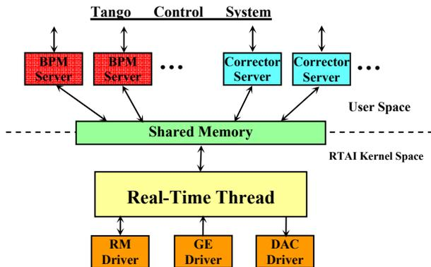
Figure 1: Software architecture of a global feedback local station.
