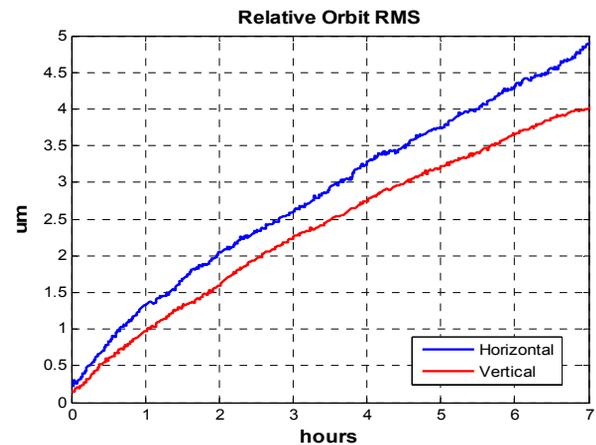
Figure 4: Orbit error *rms* with respect to a reference orbit with feedback on in a time period of 7 hours after injection and energy ramping to 2 GeV.
