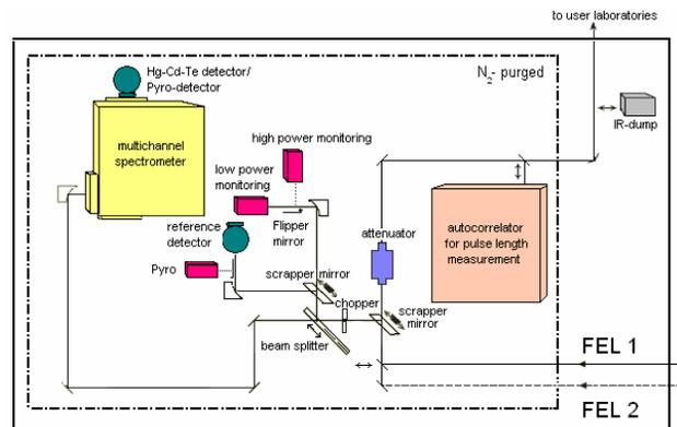
Figure 2: The optical components and devices on the diagnostic table.
