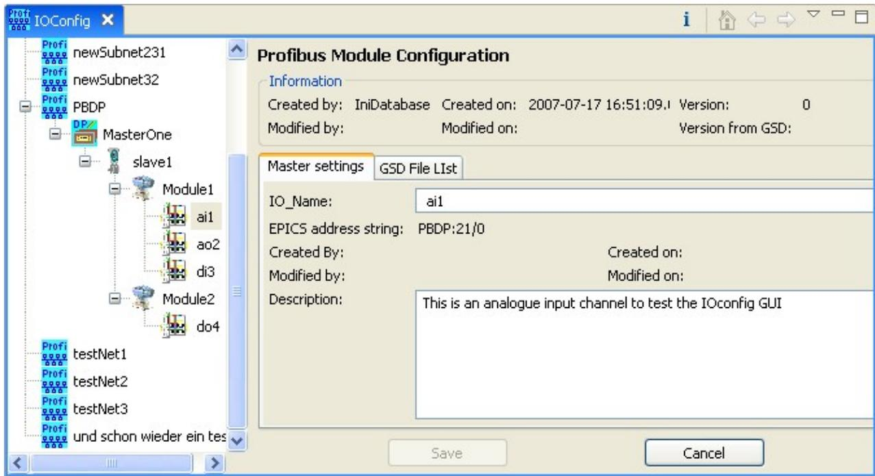
Figure 4: CSS view on the field bus tree (left) and the property window for the selected object (right).
