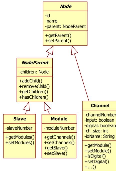
Figure 3: Schematic view of classes representing the field bus model. Slave, module and channel are specific to the Profibus field bus.
