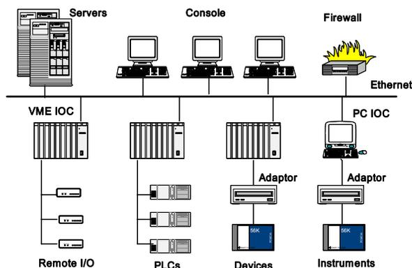
Figure 1 Architecture of BEPCII control system.
