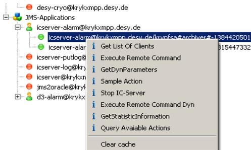
Figure 4: CSS instances with remote actions
