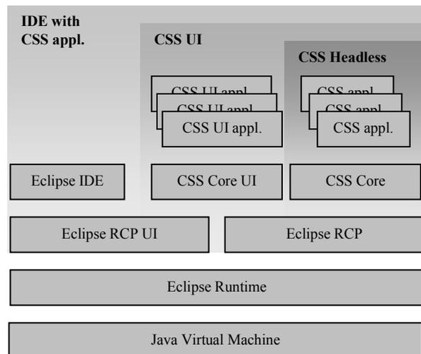
Figure 2: Architecture of Eclipse IDE and CSS
