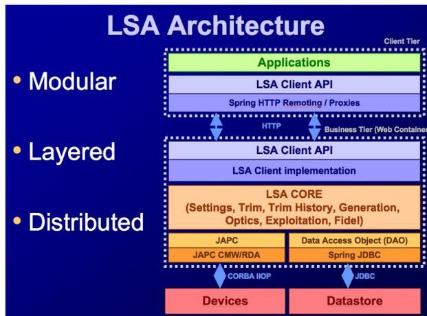
Figure 6: The LSA architecture.
