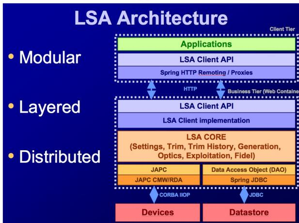
Figure 6: The LSA architecture.
