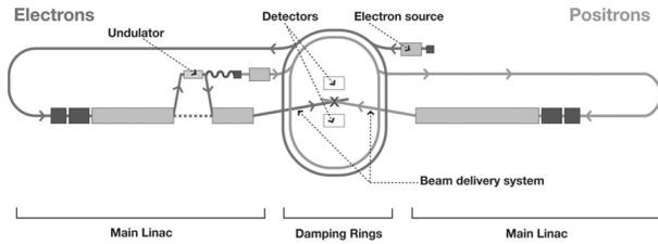
Figure 6: ILC Layout in the Reference Design Report
