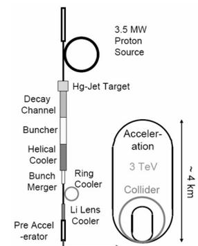
Figure 8: Layout of a Muon Collider
