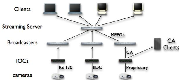
Figure 2: Image Acquisition and Streaming Video
