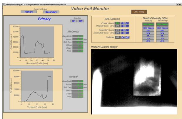
Figure 1: Video Foil Monitor console display.
