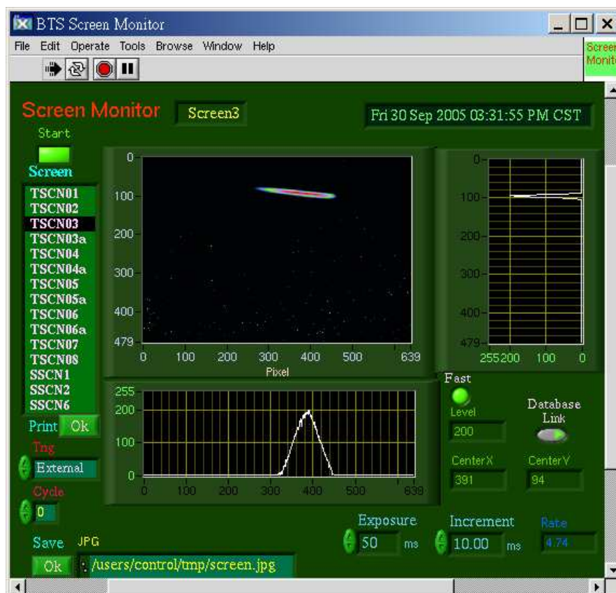
Figure 2: The control panel of screen monitor in the console.
