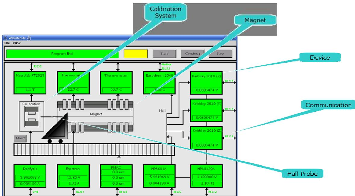
Figure 5: Main screen for controlling the magnetic measurement bench.
