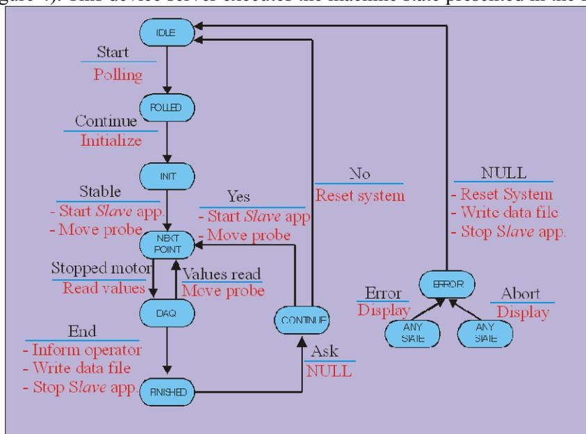
Figure 6: Magnetic measurement point-by-point state machine.
