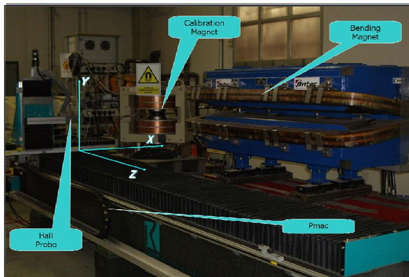
Figure 2: The magnetic measurement bench.
