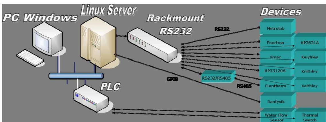
Figure 3: Hardware architecture for the magnetic measurement bench.
