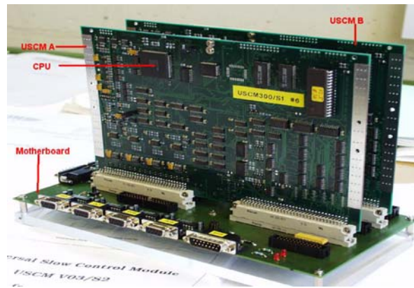
Figure 2: A pair of USCMs mounted on a special prototyping motherboard. Connectors on the motherboard export all the various analog and digital control lines offered by each USCM to special test equipment.
