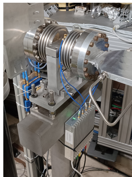
Figure 2: PTFE connected to low-gap BPMs.
