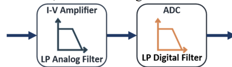
Figure 2: Analog front-end circuit block diagram.
