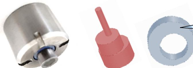
Borosilicate glass (dark blue): Inner conductor (red) with coaxial asymmetry → HOM power reduction & spectral spreading
