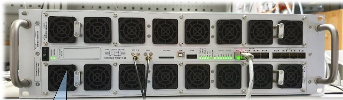
Generic 19" back-end (AMD/Xilinx **Zynq UltrasCSCale+ MPSoC**), also used in SwissFEL (-> IBIC'22 TUP12)
