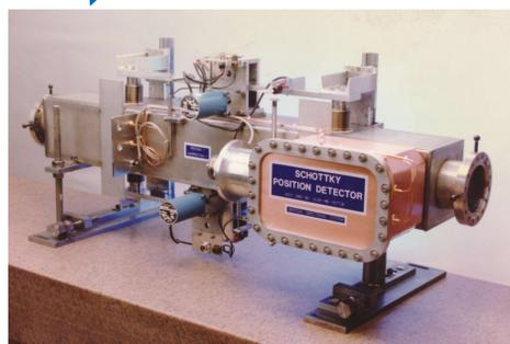
Vertical Pickup with Resonator
