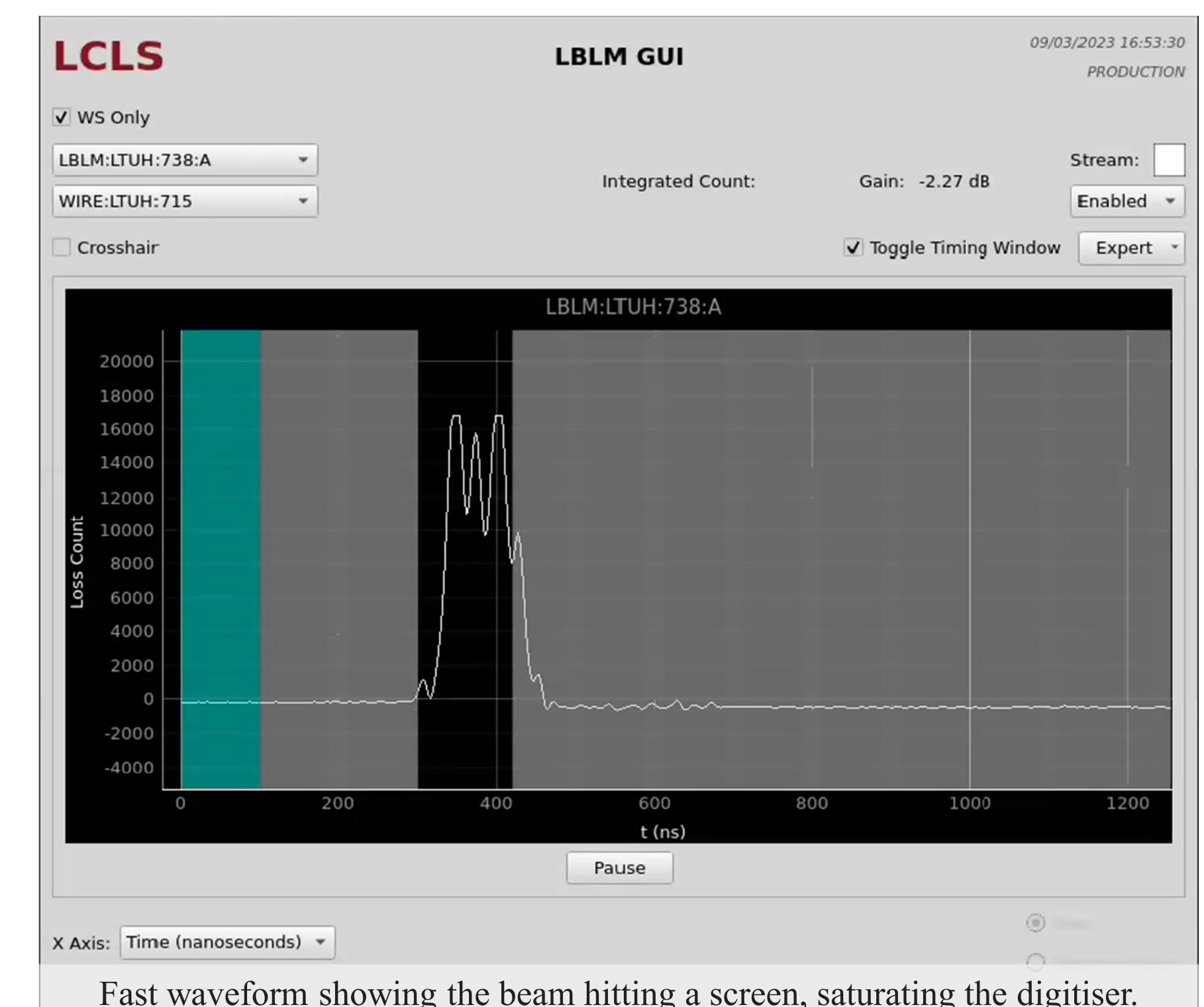
Fast waveform showing the beam hitting a screen, saturating the digitiser.
