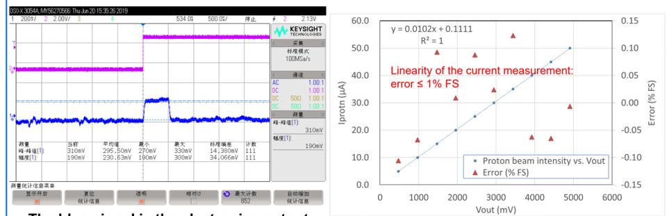
The blue signal is the electronics output with 1 uA calibrated input current.
