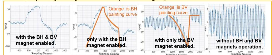
The main contribution of interference is from BH, followed by BV, which has a high similarity to the current curve of the power supply during the beam injection in the phase space painting mode.
