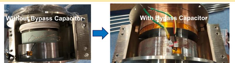
A bypass capacitor over the ceramic gap was built in the APEP-CT sensor.
