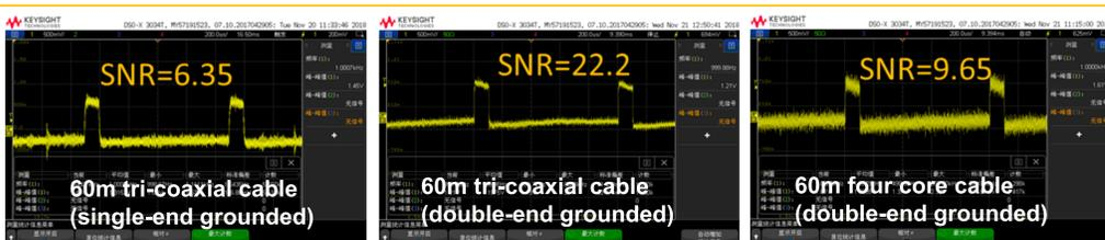
After the multi-point grounding test, it was found that outermost layer of triaxial cable was grounded to the vacuum pipeline at the sensor end, and the electronic end was grounded to cabinet ground to achieve the best effect.
