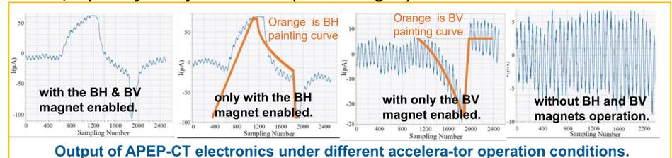
The main contribution of interference is from BH, followed by BV, which has a high similarity to the current curve of the power supply during the beam injection in the phase space painting mode.
