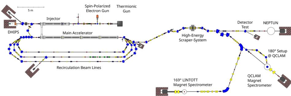
Floorplan of the S-DALINAC. To investigate fission reactions of actinides and their dependence on the excitation energy of the nucleus, electron-induced fission will be employed at the QCLAM magnetic spectrometer. The electron beam will be delivered by the S-DALINAC with a beam current of  $3 \mu\text{A}$ , a frequency of 2.997 GHz, electron energies of the order of 100 MeV and a  $3\sigma$  beam spot size smaller than 1 mm at the electrofission interaction point.
