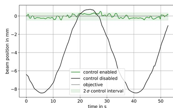
First test of a beam stabilization with a simulated beam shift (steerer), a correction steerer and a PID controller by monitoring a downstream located beryllium oxide screen. The correction magnet kept the center beam position within a  $2\sigma$ -interval of ca. 0.8 mm. It is planned to test supervised learning agents as an alternative to traditional PID controllers.
