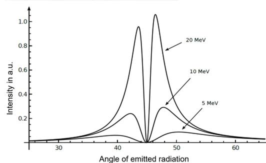
Backwards angular distribution of OTR at a  $45^\circ$  tilted diagnose screen for several beam energies. The resolution and frequency of the transverse beam profile signal only depends on the OTR intensity and both the camera resolution and frame rate.
