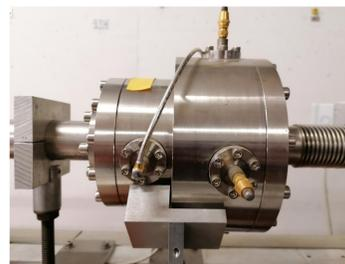
Left: Image of an in-house developed cavity beam position and phase monitor. Right: Test of this monitor for a beam current of 500 nA. Beam positions with an increment of 1 mm can be resolved.
