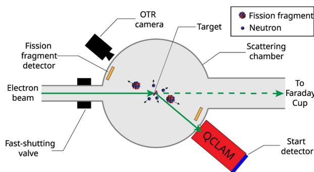
Design of the electrofission setup at the QCLAM. After its interaction with an electron the target nuclei can decay via fission. An accurate description of this process, which is not available up to date, requires the measurement of both fission fragments in coincidence.
