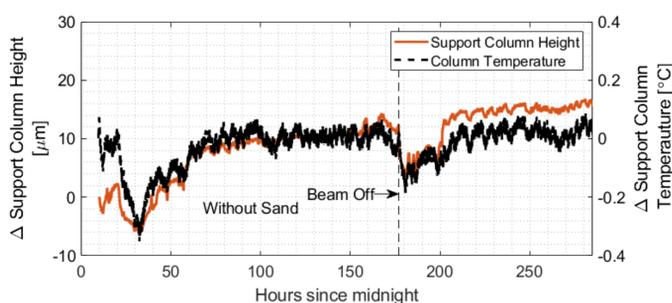
The change in the support column height and the average column temperature measured with (top) and without (bottom) sand filling the column
