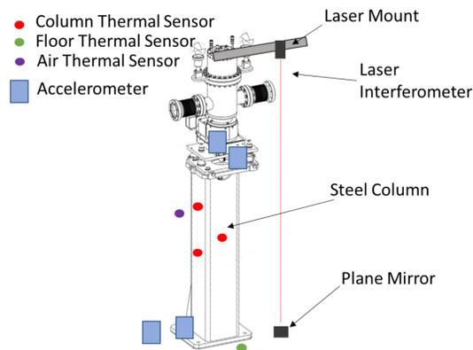
A drawing of the XBPM and its support column, with the locations of the different devices.
