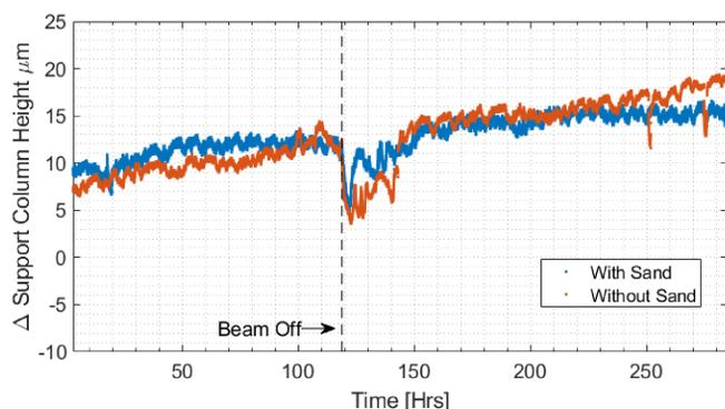
The change in the support column height measured with and without sand filling the column
