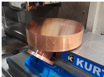
Figure 9: Photograph of the mirror and polishing fixture during machine lapping.
