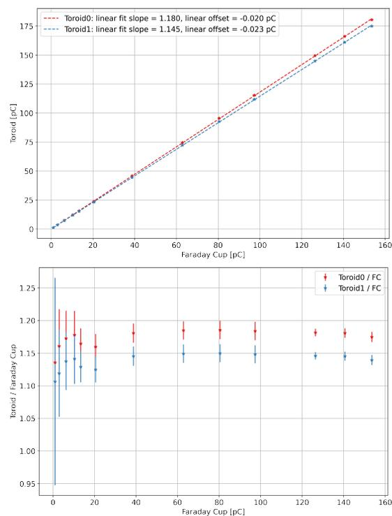
Figure 6: Linearity of the Toroids.
