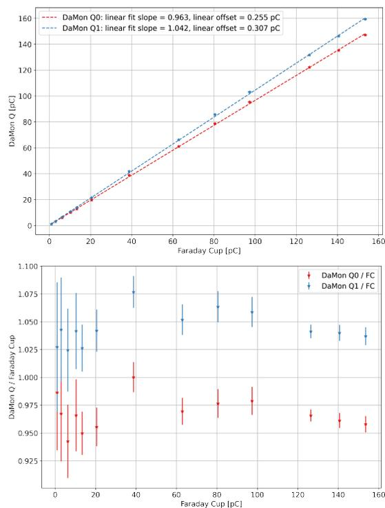
Figure 5: Linearity of the DaMon *Q* channel.
