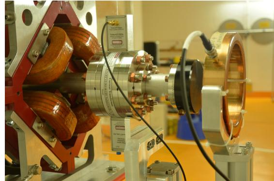
Figure 3: T-ICT (left) installed in vacuum, output window of the beam line (black cover in the middle) and the in-air ICT (copper colored toroidal shape on the right). The electrons are used for in-air experiments direct downstream the in-air ICT.
