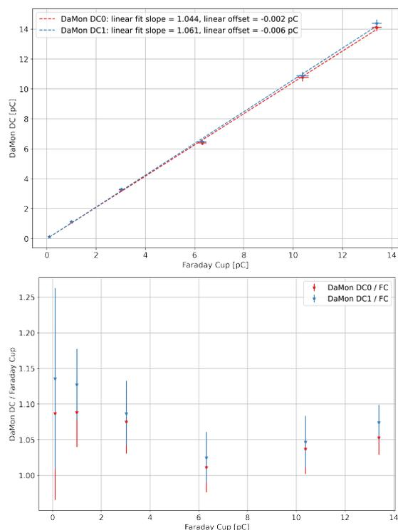
Figure 4: Linearity of the DaMon *DC* channel.
