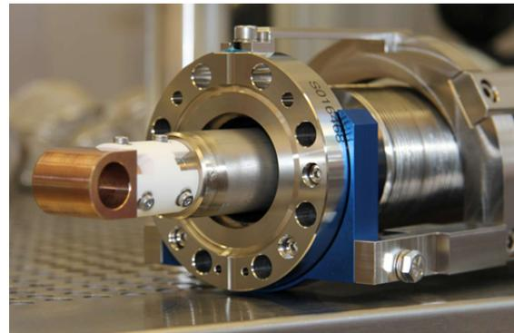
Figure 1: New Faraday Cup mounted with ceramic spacer on a mover rod.
