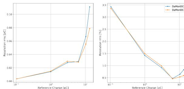
Figure 9: Absolute and relative resolution of the DaMon DC channels in the range of 0.1 pC to 13 pC.
