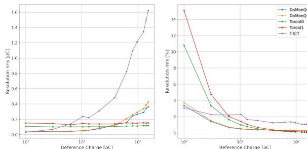
Figure 10: Absolute and relative resolution of DaMon Q channels, Toroids and T-ICT, each in the range of 1 pC to 153 pC.
