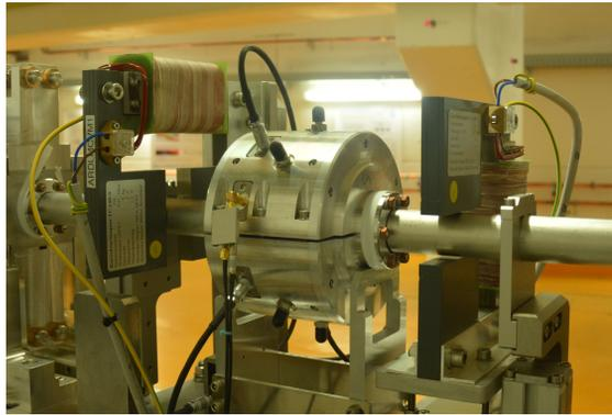
Figure 2: Toroid installed in the ARES accelerator. The diameter of the beam pipe is 34 mm, the length of the Toroid (flange to flange) is 150 mm.
