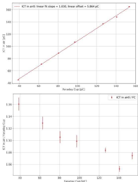
Figure 8: Top: measured charge of the in air ICT as a function of Faraday Cup charge; below the ratio of the in-air ICT to Faraday Cup charge as a function of Faraday Cup charge. Both in the range of 30 pC to 153 pC.
