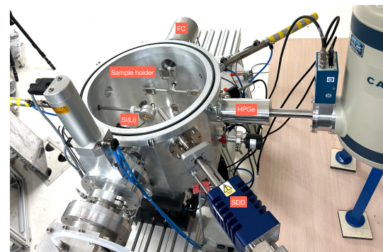
Figure 1: Irradiation system and detector placement.
