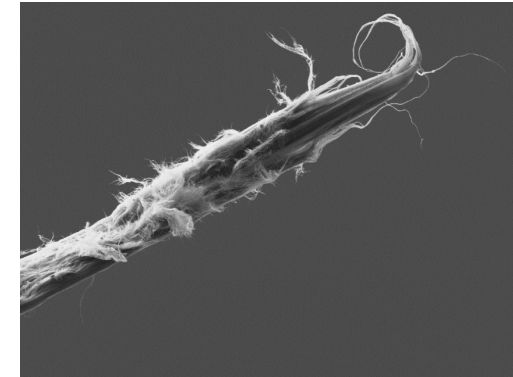
Fracture area of a thick yarn
