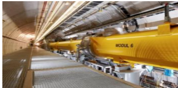
TESLA type superconducting accelerating modules 1.3 GHz
