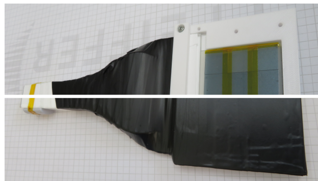
Figure 7: Photographs of the ZnO-based multi-tile scintillator detector. The upper photograph shows a part of the multi-tile assembly, while the bottom half is a photograph of the detector wrapped with PTFE and black tape.
