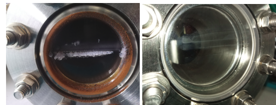
Figure 3: Pictures of the UHV Fused Silica window. Left: after 10 years of operation. Right: after 2 years of operation.
